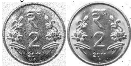
Fig. 1: Gaussian and salt-and-pepper noise affected images.
